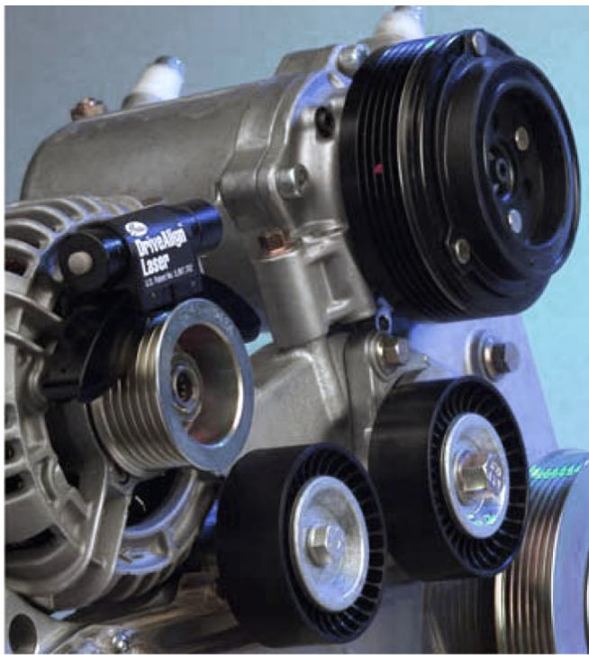
Use Gates DriveAlign® Laser Alignment Tool (Part #91006) to quickly identify pulley misalignment.
